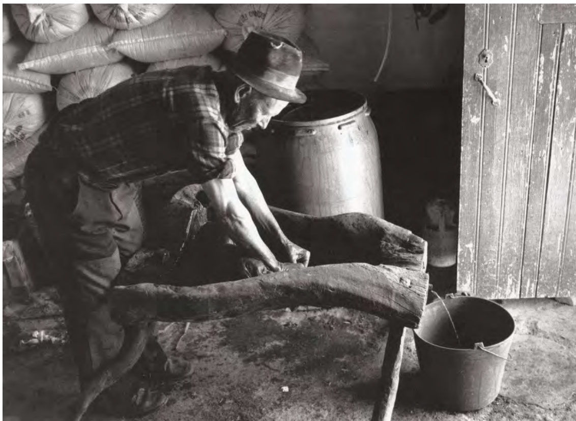
FIGURE 5 The “burra” or manual press typical of the Algarve mountains.
